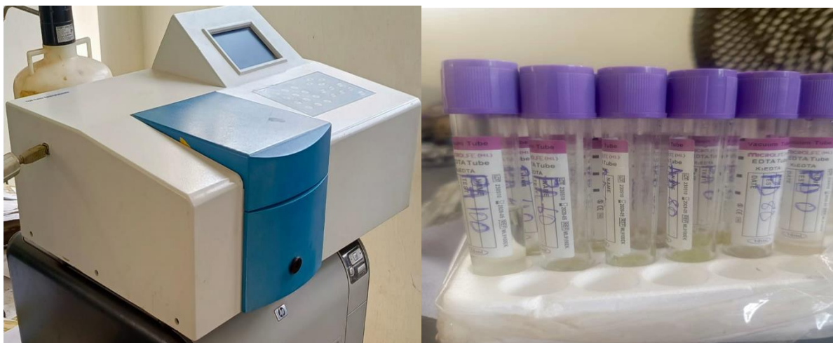
Figure 1: Shanghai INESA Model 723N UV-Vis Spectrophotometer with Plastic Stripes Containing Prepared Samples for Analysis
