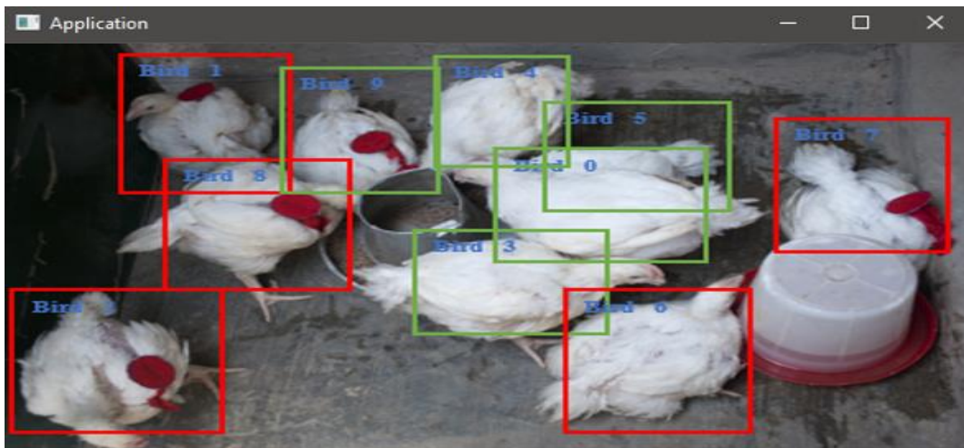
Figure 4: Results of MobileNetSSD model for tracking and detection of broilers in farm B
