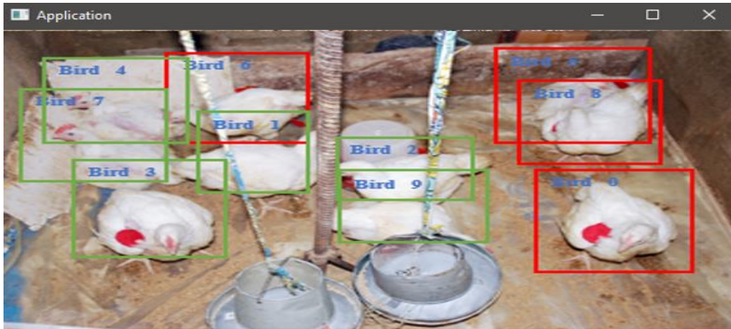
Figure 3: Results of MobileNetSSD model for tracking and detection of broilers in farm A
